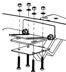
Attach the Hinges to the frame using the supplied 4mm nuts, bolts and washers so the face plate protrudes around 10mm from the frame. The exact depth will be adjusted later. Just tighten the two bolts diagonal to one another for now.
