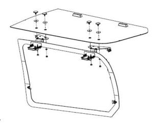
Once all four pan heads are in place and secure, check that the door doesn't touch the car when opening and closing. If there is any touching, adjust the door accordingly before attaching the gas struts.
